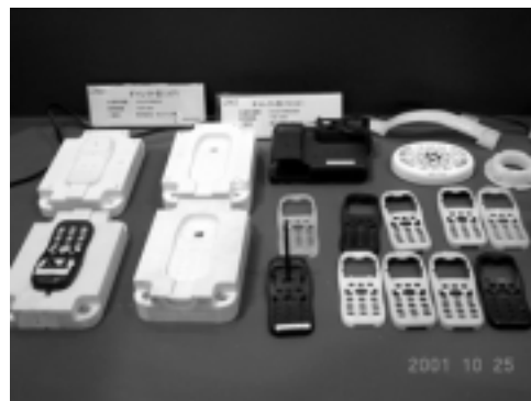
Figure-6. Injection molding die of TSR-2081 and its injected ABS product.
